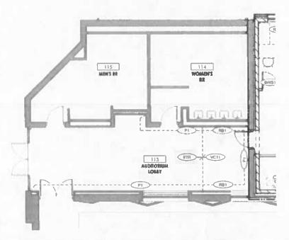
Interior Finish Plan Sheet A2.2 – Indicates for the carpet in the auditorium to the left of the old coat room to remain. PR#004 has requested a credit for the flooring in the auditorium lobby and there is not a credit to provide as the flooring contractor did not pick up flooring for this area.
