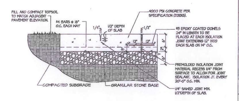
8" HEAVY DUTY CONCRETE PAVEMENT AT DUMPSTER PAD SCALE : N.T.S.
