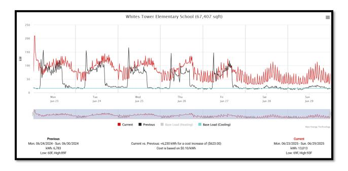
High humidity levels at White's Tower Elementary have forced the increased use of cooling to dehumidify. High humidity levels a re a real concern in areas with carpet, specifically in classrooms not being utilized during summer months. Upcoming renovation project will address the remaining carpet in classrooms.
