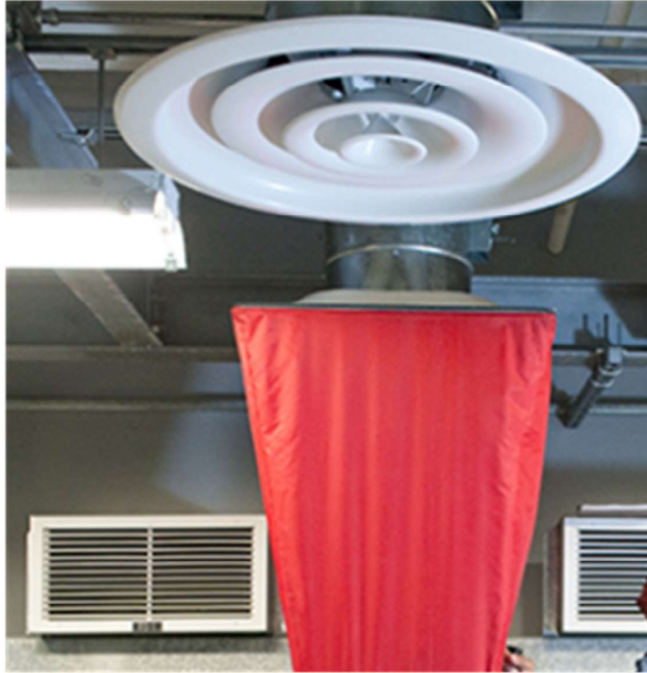
Figure 1 Testing and balancing of HVAC airside components.
