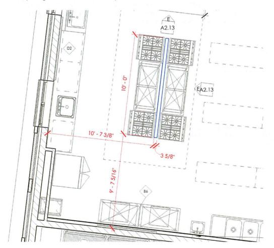
2. Provide pricing for 2 stainless steel chases, floor to ceiling in height, in the locations below. Field verify chase size for gas line requirements.
