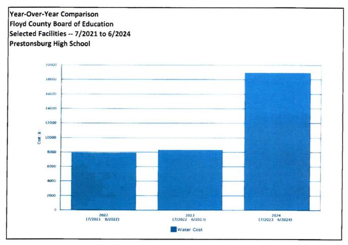
Increase 2024 due to float sticking in the cooling tower pit and overflowed and pipes freezing and bursting in the football fieldhouse.
