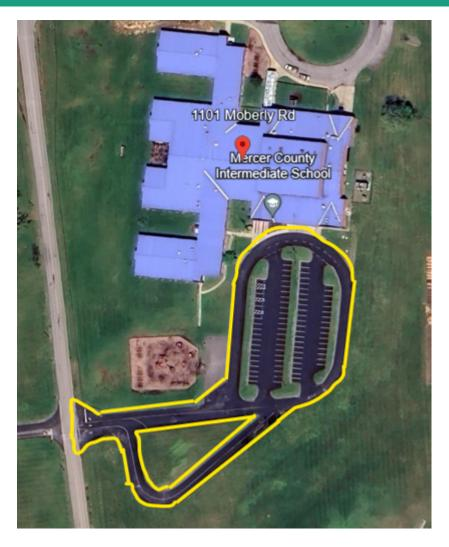
Services Included: Crack Filling, Seal Coating, and Re-Striping of the area marked in Yellow
