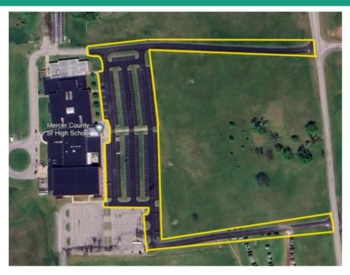
Services Included: Crack Filling, Seal Coating, and Re-Striping of the area marked in Yellow
