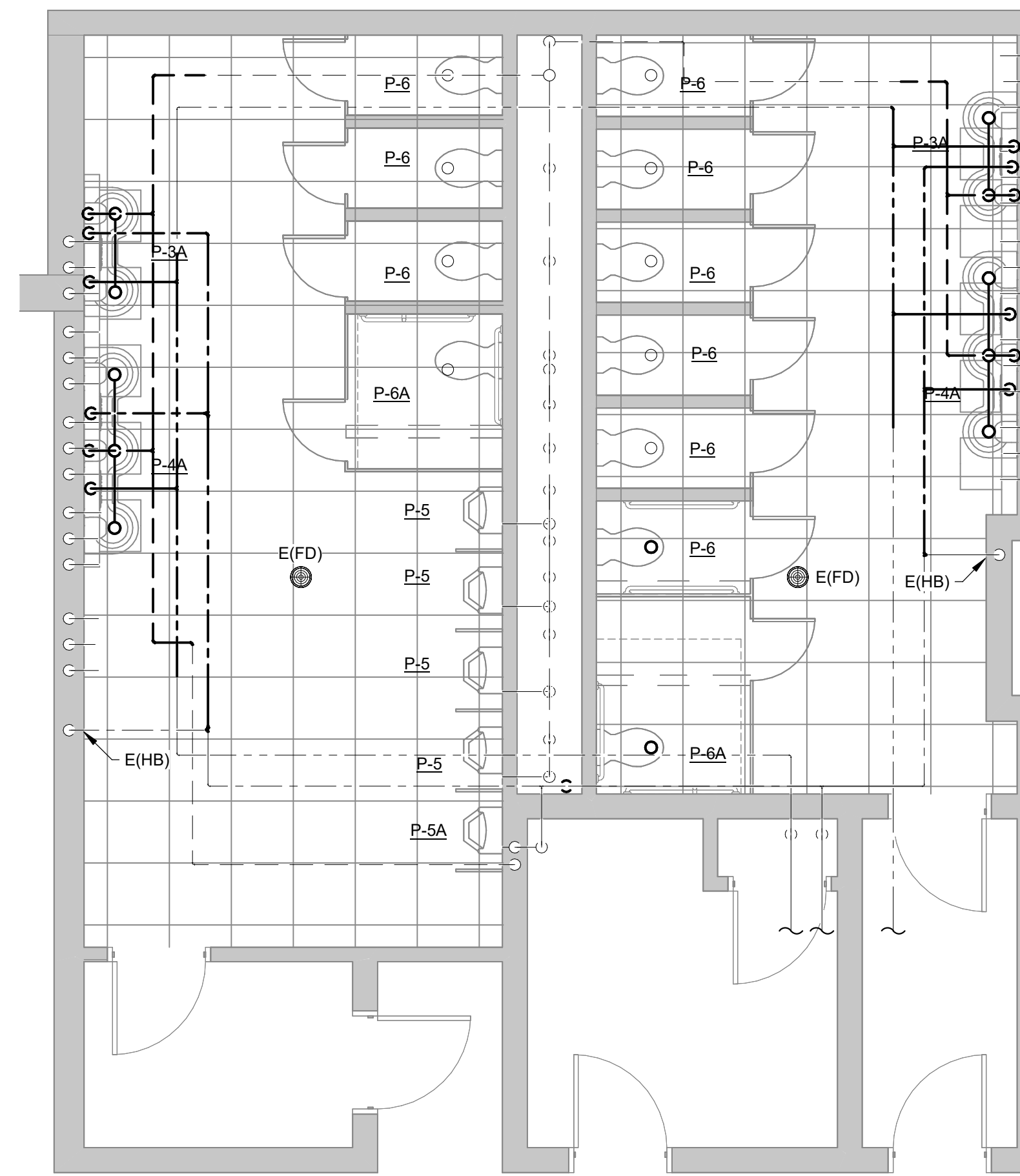
STEVENSON ELEMENTARY SCHOOL RESTROOM 135 ABOVE SLAB NEW WORK PLUMBING PLAN
