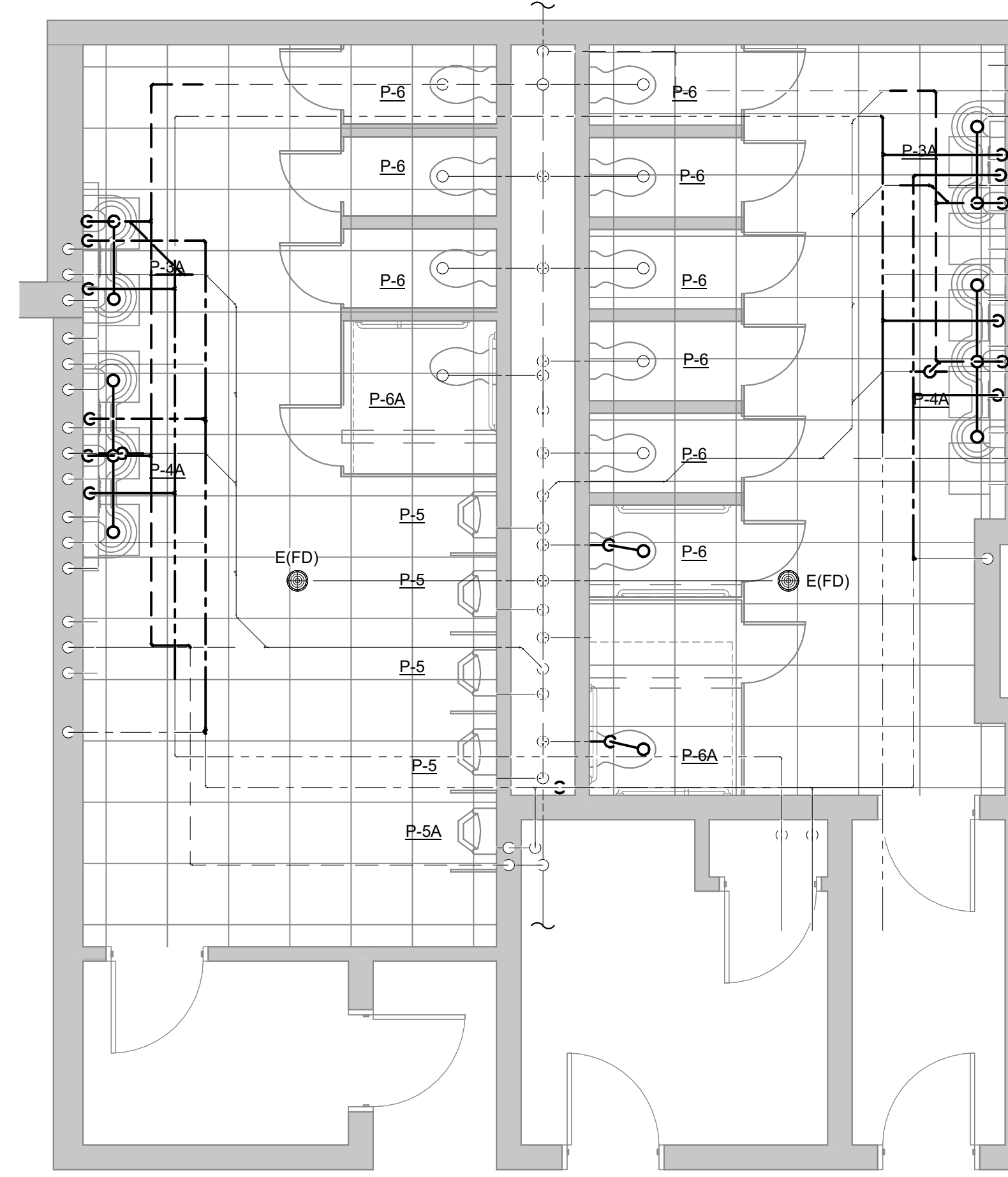
STEVENSON ELEMENTARY SCHOOL RESTROOM 135 UNDER SLAB NEW WORK PLUMBING PLAN
