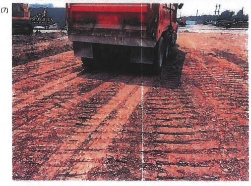
(Test #4) Proofroll with loaded truck showing material to be stiff with little to no movement. (Light duty pavement design side)
