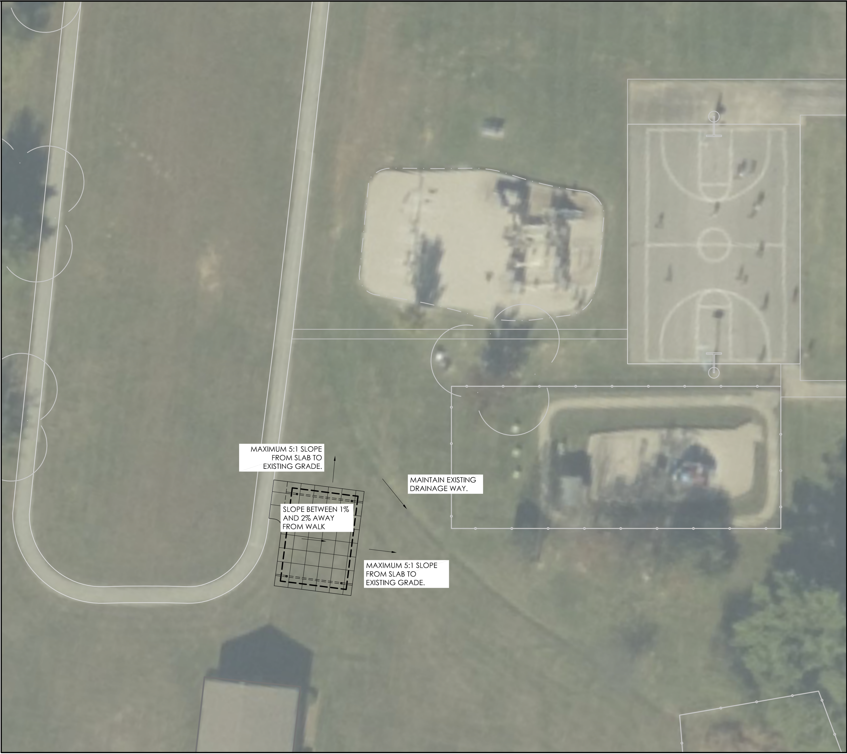
SITE GRADING AND DRAINAGE PLAN - GLASSCOCK ELEMENTARY
