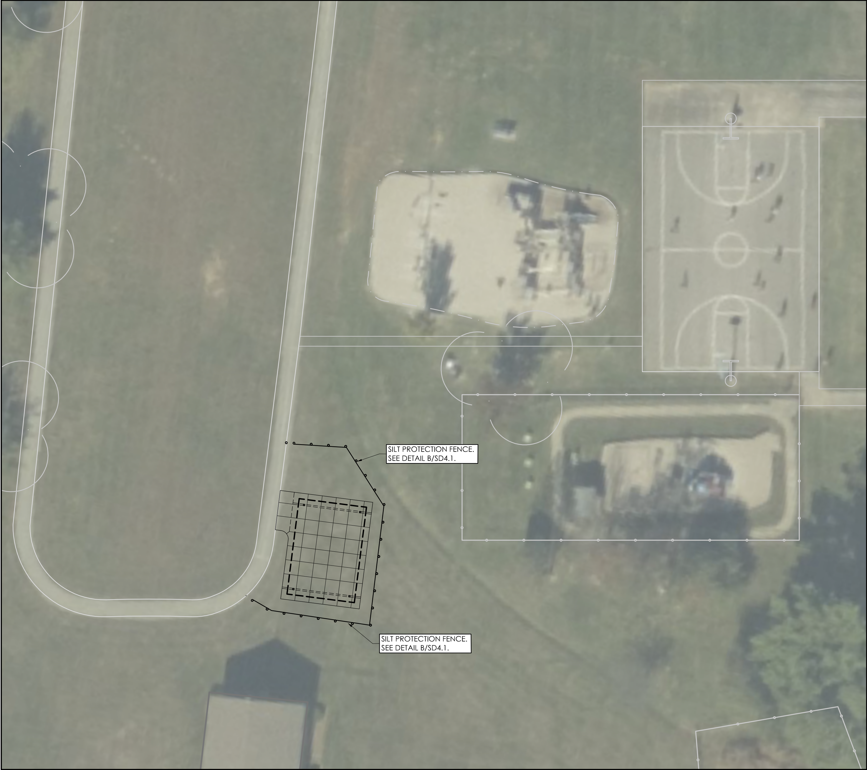
EROSION POLLUTION SEDIMENT CONTROL PLAN - GLASSCOCK ELEMENTARY SCALE: 1"=20'
