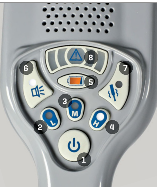
Optical indication proportional to the radioactive substance signal strength.
