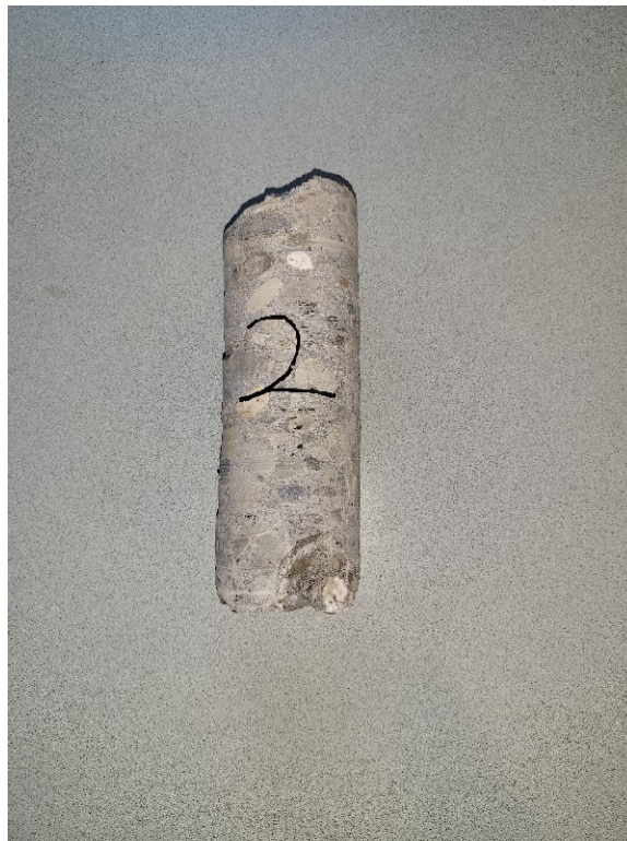
Photo 6: The second core was taken in the middle of the seating. The top of the core is soft similar to the first but does penetrate the depth of the concrete more than two inches.
