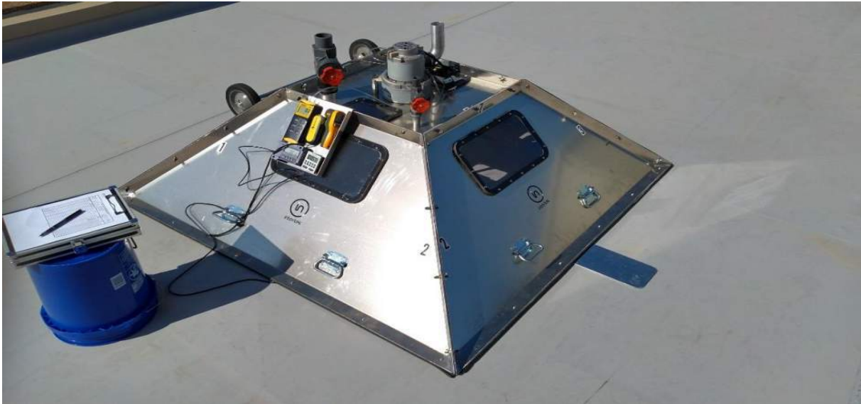
Photo 1: Typical test equipment set-up with 5'x5' negative pressure bell chamber. (Stock photograph)
