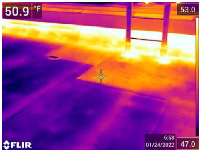
An area of wet insulation.
