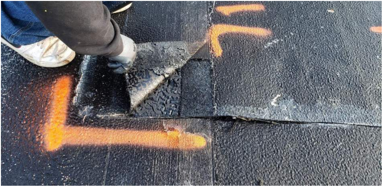
Photo 7: T-1 – Mode of Failure noted between cap sheet and inter-ply membranes, water evident between roof membranes.
