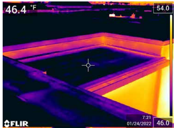
Infrared overview photo of the roof system. No anomalies identified.
