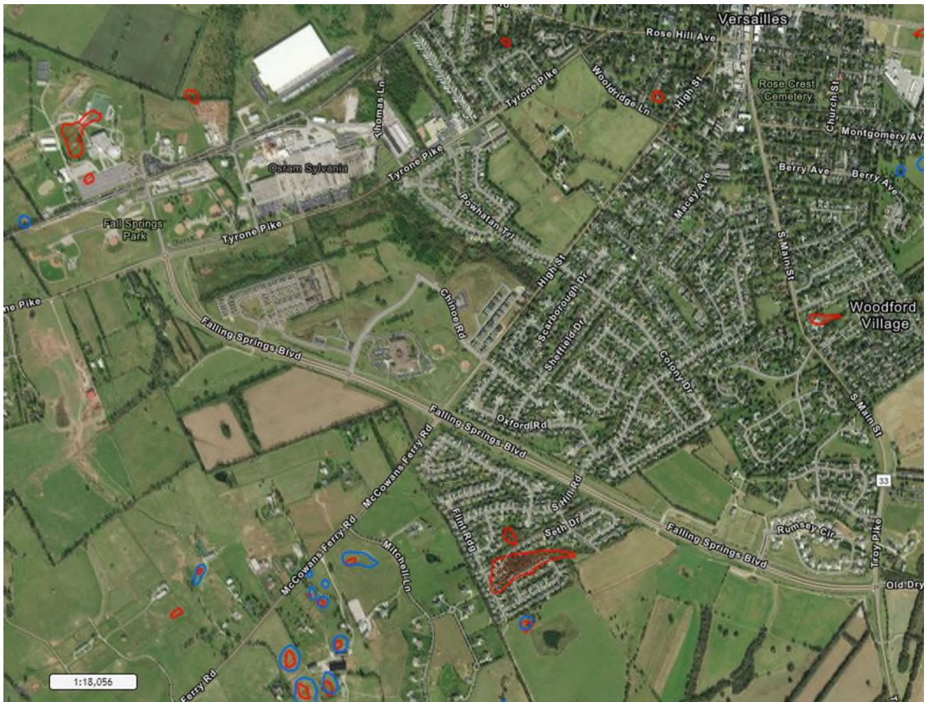
Figure 2- Mapped Sinkholes Outlined in Red (source: Kentucky Geological Survey)
