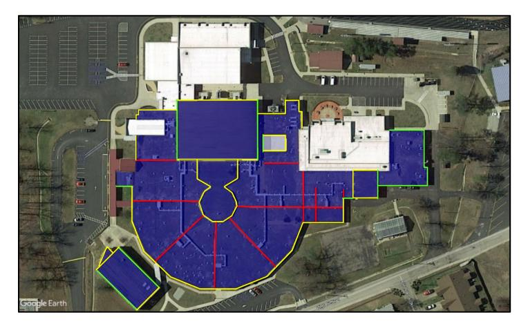
Blue Area - Indicates area of reroof Yellow Line - Indicates area of new foam stop. Green Line - Indicates area of new gutter. Red Line - Indicates area of new expansion joint.
