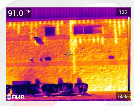
IMAGING OF NEWLY GROUTED CMU WALLS WILL PROVIDE PROPER INSTALLATION AND ALSO LOCATE DEFICIENCIES. IF DEFICIENCIES ARE LOCATED THEN THEY CAN EASILY BE REPAIRED WITHOUT THE DESTRUCTION OF EXCESSIVE MATERIALS. THIS IS A MUST TO HAVE AS A QC CONFIRMATION PRIOR TO INSTALLING ROOF SYSTEMS OR THE DEFICIENCIES MAY RESULT IN SHORT OR LONG TERM FAILURE.
