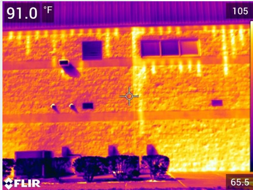
IMAGING OF NEWLY GROUTED CMU WALLS WILL PROVIDE PROPER INSTALLATION AND ALSO LOCATE DEFICIENCIES. IF DEFICIENCIES ARE LOCATED THEN THEY CAN EASILY BE REPAIRED WITHOUT THE DESTRUCTION OF EXCESSIVE MATERIALS. THIS IS A MUST TO HAVE AS A QC CONFIRMATION PRIOR TO INSTALLING ROOF SYSTEMS OR THE DEFICIENCIES MAY RESULT IN SHORT OR LONG TERM FAILURE.
