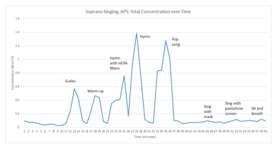
Playing wind instruments, singing, and theatrical voice releases airborne particles (aerosol). These particles are of the size range that may transmit the COVID-19 virus. Performing with mask and bell cover reduces emissions.
