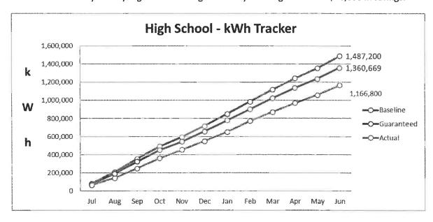
Figure 7 Electrical consumption tracker showing the actual performance beating the guarantee.
