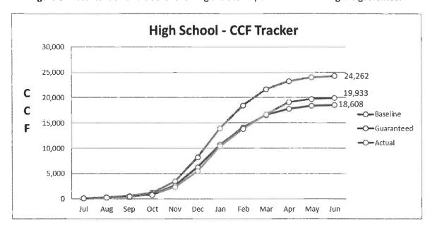
Figure 9: Natural Gas tracker showing the actual performance compared to the guarantee.
