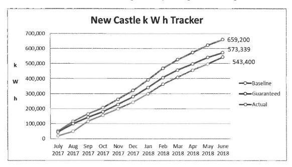
Figure 10: Electrical consumption tracker showing the actual performance beating the guarantee.
