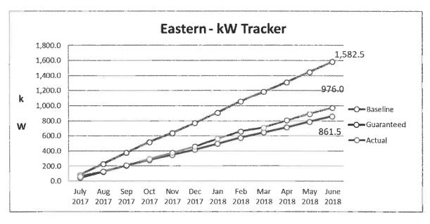
Figure 2 Electrical Demand Tracker showing the actual performance compared to the guarantee.
