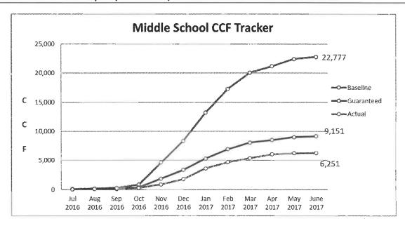
Figure 5 Natural Gas tracker showing the actual performance beating the guarantee by more than 30%.
