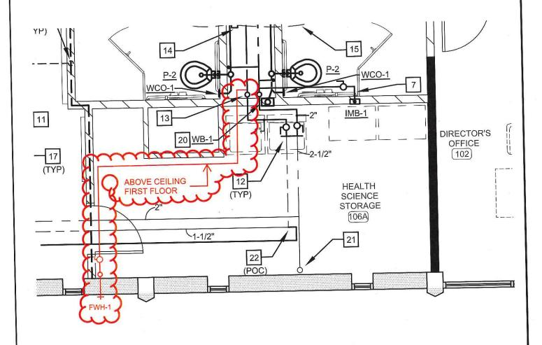
WOODFORD MODEL NO. 67 AUTOMATIC DRAINING WALL HYDRANT WITH WHEEL OPERATION, COVER AND POLISHED BRONZE FREEZEPROOF WALL FWH-1 FINISH. HYDRANT
